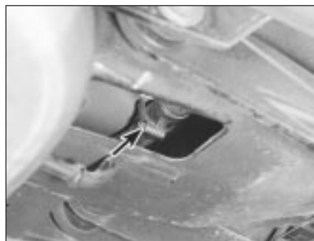
10.7A Fuel filler vent hose clamp (arrowed) is accessible through right-hand side aperture in rear suspension crossmember on Saloon and Hatchback models . . .
