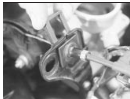
5.3 Removing clip securing accelerator cable to throttle housing bracket
