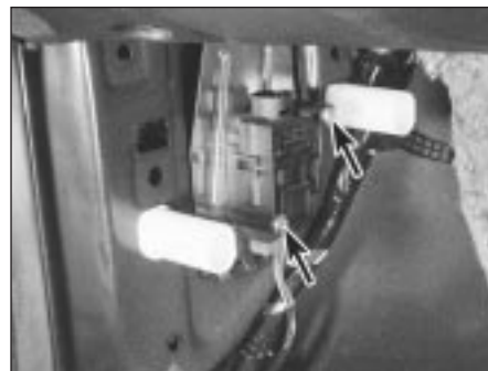
13.3 Fuel cut-off switch retaining screws (arrowed)
