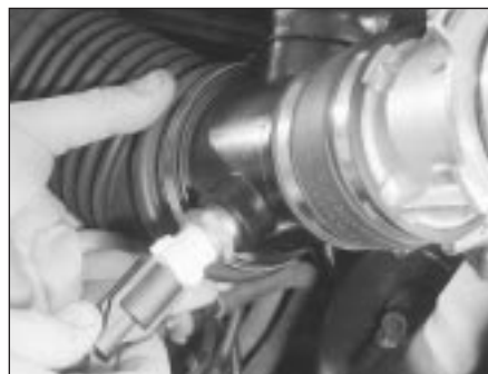
4.7 Unplugging intake air temperature sensor's electrical connector
