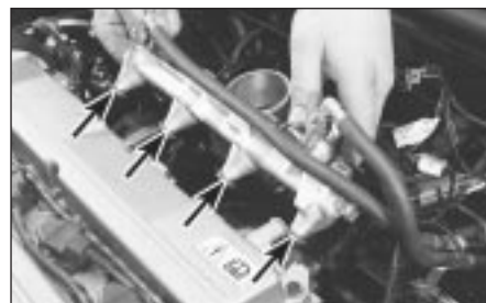
16.19B . . . and withdraw fuel rail with injectors and pressure regulator - renew nose seals (arrowed) whenever rail is disturbed
