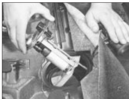
9.7A Removing fuel pump/fuel gauge sender unit - take care not to bend float arm, and note how it is fitted on spring-loaded extension
