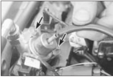
16.29 Disconnect vacuum hose, and unscrew bolts (arrowed) to withdraw fuel pressure regulator
