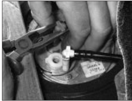
9.5 If fuel couplings are difficult to release, use pliers and a block of wood as shown to prise pipe end out of union - be careful not to damage pipes or unions
