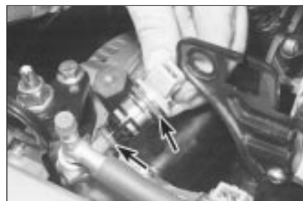
16.12B . . . and removed individually if required, but it is better to remove them with the fuel rail, if servicing is necessary. O-ring seals (arrowed) must be renewed whenever injector is removed
