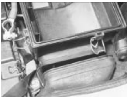
4.5 Ensure air filter housing intake mouth is fully engaged inside connector sleeve
