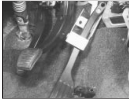
7.2 Removing the accelerator pedal assembly
