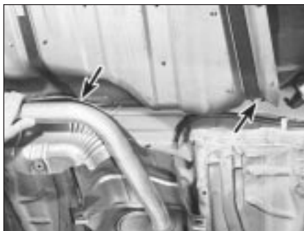
10.8 Exhaust system must be lowered and heat shield removed to enable fuel tank removal - arrows show location of retaining strap front bolts
