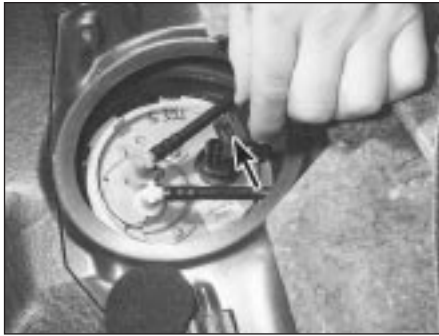
9.4 Unplugging the fuel pump/fuel gauge sender unit electrical connector (arrowed)
