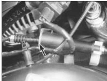
5.9 Location of accelerator cable adjuster - remove metal clip (arrowed) to enable adjustment to be made
