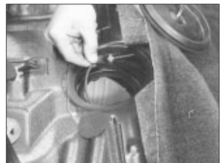
9.7B Fuel pump/fuel gauge sender unit's sealing ring must be renewed whenever it is disturbed
