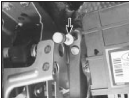
5.4 Pull the accelerator cable end fitting (arrowed) out of the pedal
