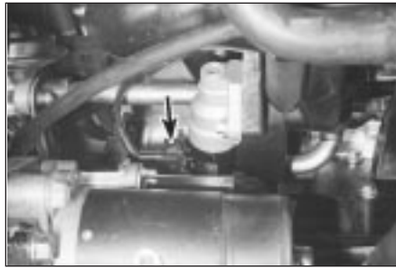
16.33 Access to idle speed control valve is from underneath vehicle - unplug electrical connector (arrowed) to check valve
