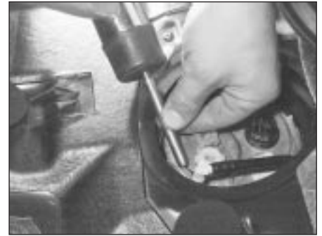
9.6 Fuel pump/fuel gauge sender unit's retaining ring can be released using ordinary tools as shown. Correct service tool will probably be required on refitting
