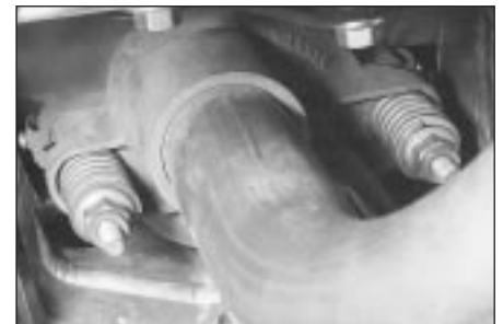
17.5 Tighten exhaust system front downpipe-to-manifold nuts as described - do not overtighten them
